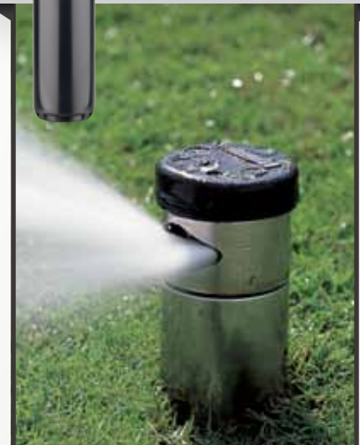
I-40-06: Overall height: 10 1/4" Pop-up height: 6" Exposed diameter: 2" Inlet size: 1" female NPT
