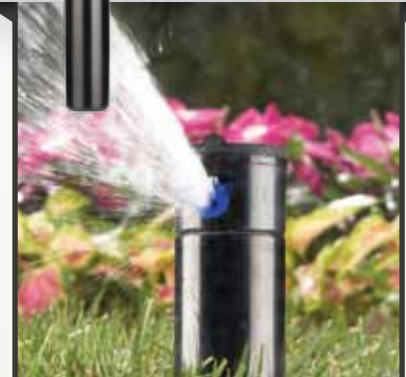
PGP-12: Overall height: 17" Pop-up height: 12" Exposed diameter: 1¾" Inlet size: ¾" female NPT
